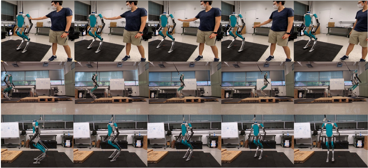
Fig. 6: Tile plots of Digit recovering from a external push (top), blind walking on stairs (centre), and turning in place as per command (bottom) using the learned linear policies.
